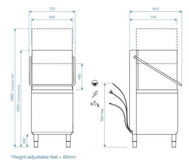
Pumped waste into upstand, maximum height 700mm
